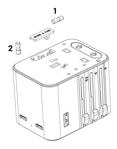
This appliance is equipped with a 10A overload fuse. In the event of an overload, the fuse will automatically disconnect. Replace it with the provided spare fuse.
