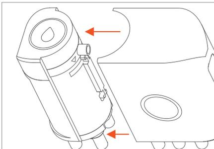
1. Remove the tank cap, then gently pinch the tank and pull it outward to detach it from the main unit.
