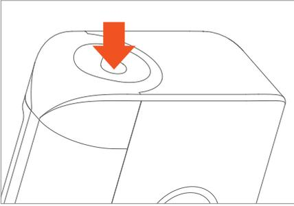
**5.** Press the button to dispense 1 ml of solution into the direct-use tank. Release the button once the tank is filled.
