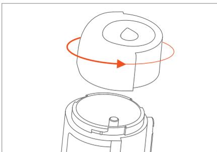
2. Twist the tank cap counterclockwise from CLOSE to OPEN.
