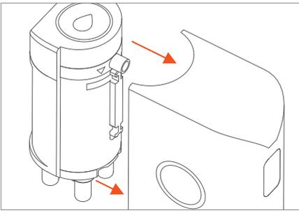
**4.** Reinstall the tank onto the main unit. Gently press it into place until a 'click' sound is heard, indicating proper attachment.
